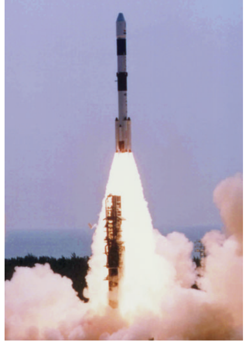
The force of the gases pushes downward at the same time that the gases push the rocket upwards.
