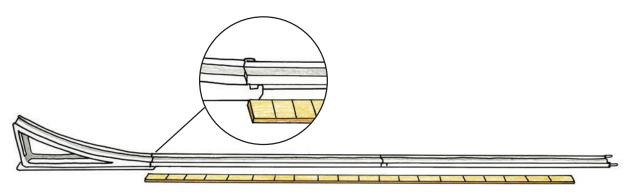
2. Use the meterstick, masking tape, and marker to measure and mark the beginning and end of the first 100 cm of the level part of the track. Make sure to place the tape next to the track instead of directly on the track.
