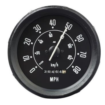
This car speedometer shows speed in miles per hour and in kilometers per hour. Kilometers per hour is the speed unit commonly used in other countries.
